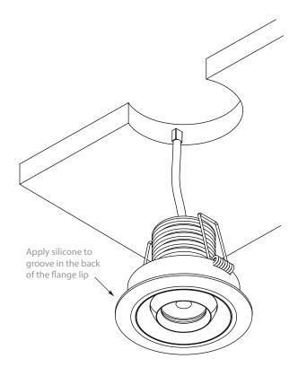
Draw power supply cable down through the cut hole and make a good electrical connection with the fixture input cables. See diagram for correct wiring. Be sure to leave extra length to allow the fixture to be removed from the ceiling without disconnection for servicing.
