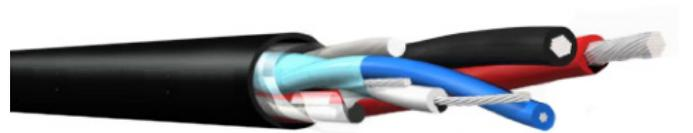
The special highly rated LuxR Hybrid DMX Cable 2x 1mm² tinned power cores, 12-24V DC Data +, Data -, Data Ground (Drain Wire for shield) of the correct impedance
