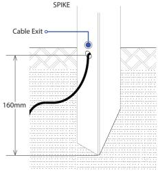
When a spike is used, push into substrate with Cable Exit above or below the ground, as desired and make water proof connection
