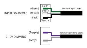
Once connections have been made fix the luminaire onto the mounting plate (check that the backplate gasket is in place) and use screws provided to secure luminaire. Make sure to use the washers supplied are fitted under the mounting screws to stop water leaking into the luminaire. If there is any possibility of water leading down the cable track, the cable entry point must be waterproof sealed. (See Fig. 2)
