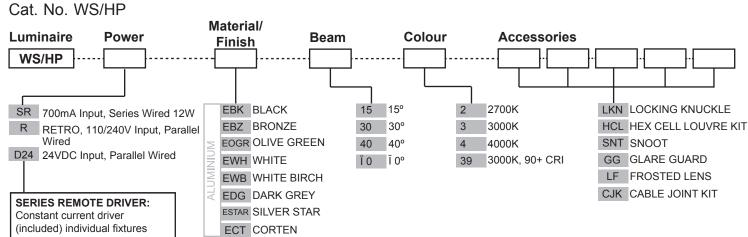
require 18vdc @ 700mA maximum. 0-10 volt dimming.
