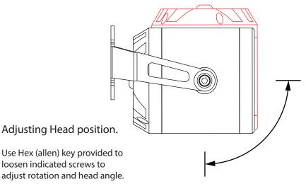
Once desired postioning is achieved tighten screws to lock in place
