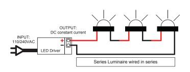
Diagrams are a guide only, wire colours and polarity may change depending on fixture and country
