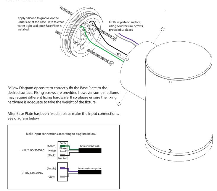
Once Wall preparations and input connections are completed. Slide the base and head over base plate. Once in position fix in place using the three grub screws.
