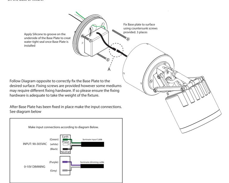
Once Wall preparations and input connections are completed. Plug driver output cable into fixture input cable (see point A on diagram). Now slide the base and head over base plate. Once in position fix in place using the three grub screws.
