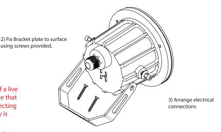
4) Refit the main Fixture body onto the bracket Taking care to reinstall the ferrules and Bolts Tighten to fix the aiming position.
