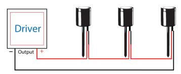
Fixture with Internal Driver Wired in Parallel
