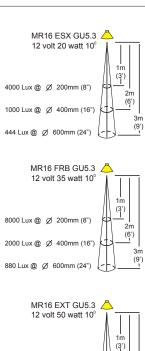
(3') | 10000 Lux @ Ø 200mm (8") 2п (6') 2500 Lux @ Ø 400mm (16") 1000 Lux @ Ø 600mm (24")
